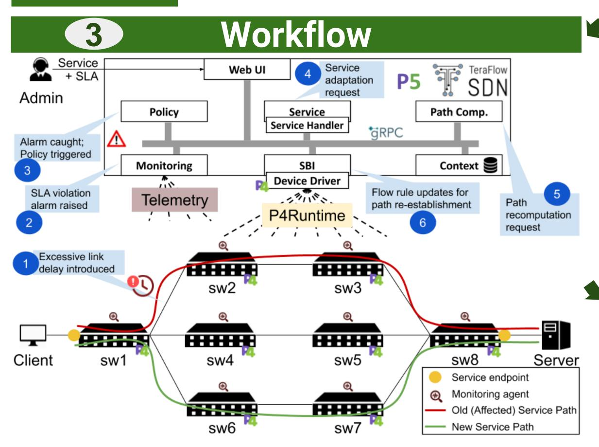
end-to-end the latency exceeds Monitoring sends an alarm to component, which requests and establishes an alternative path, through the Service and Path Computation components. This procedure takes less than 4 sec to complete from the moment of the alarm to the establishment of a new service path.
