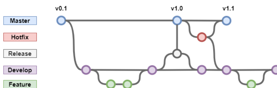
Figure 15 GitFlow graph representing an exemplary structure involving the five types of branches
